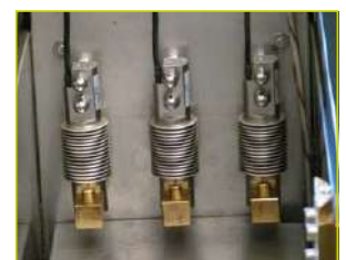
Detail: 3 load cells 500 N
